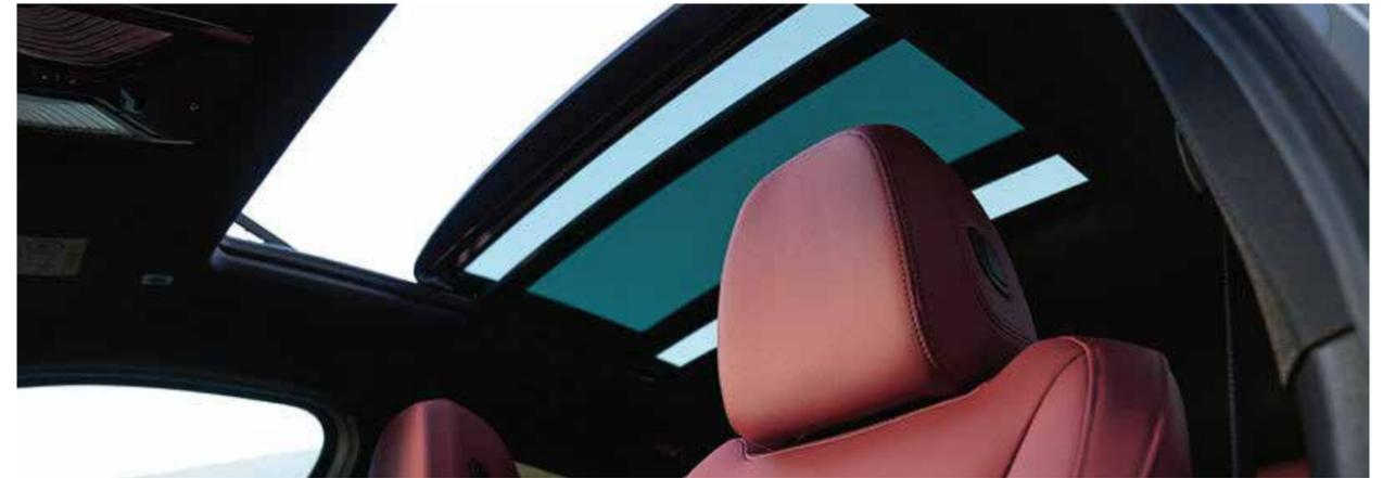
□ When open, the Panorama glass roof provides a great deal of fresh air. Closed, it creates a bright, light-flooded atmosphere in the interior. It opens and closes completely automatically at the push of a button or with the vehicle key, and is equipped with slide and lift functions, roller sunblind and wind deflector.
