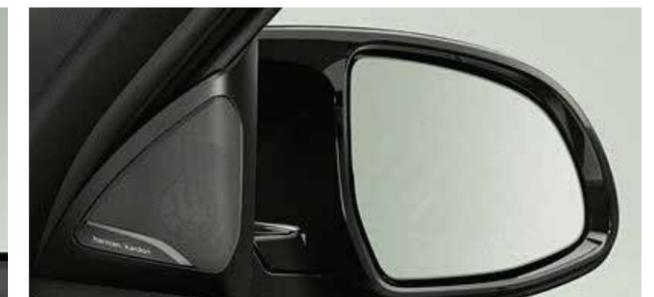
□ The tonally outstanding Harman Kardon surround sound system features a 464-watt digital amplifier, nine channels and 16 speakers. Its sophisticated sound perfectly fills the interior space. Vehicle-specific, speed-dependent equalising precisely compensates for any background driving noise.
