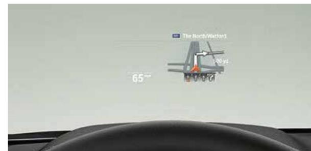
□ The full-colour BMW Head-up Display<sup>2</sup> projects all information relevant to the journey directly into the driver's field of vision, thereby allowing them to fully concentrate on driving. Information such as the current speed, navigation directions, speed limit display including no-overtaking indicator, along with telephone and entertainment lists are displayed, depending on the equipment.
