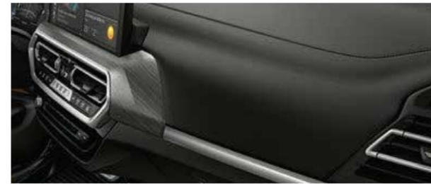
□ The Instrument panel in Sensatec lends the interior of the vehicle a highly exclusive atmosphere. The artificial leather is applied directly to a semi-rigid foam, and features an impressively soft surface. The wear-resistant material around the door panels on the front and rear features attractive double-lap seams.
