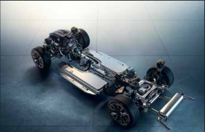
With the standard adaptive 2-axle air suspension incl. self-levelling suspension, you will also experience exceptional ride comfort and high driving dynamics.
